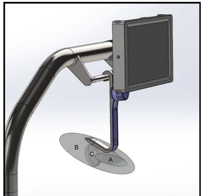
FIGURE 2. Magnified view of the CoreVista Retractor and high-definition display. The retractor can be operated with three different illumination modes (A, B, and C) for optimal illumination of different zones of the operative field as described in Table 1. Light beams from the various illumination modes are superimposed for illustrative purposes.
